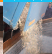
Delivery of woodchips to fuel silo
